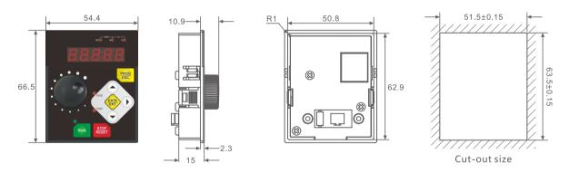
Note: This keyboard can be extended with ordinary network cable (8 cores).
