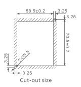
• Remote keypad(EL-OP-B2) external dimensions and installation dimensions (Unit : mm)
